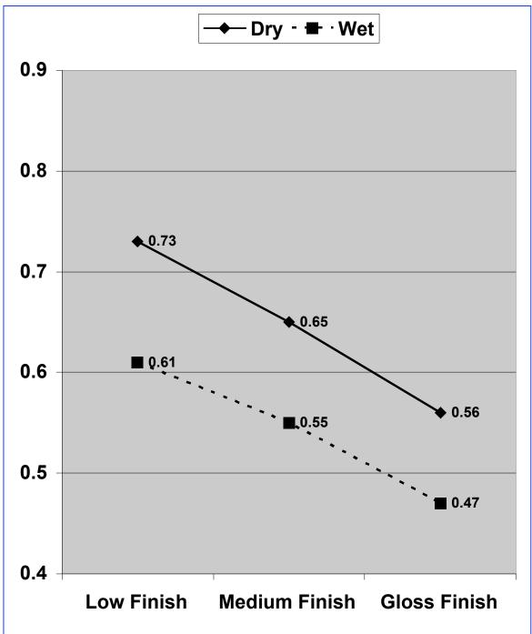
\*NOTE – According to the ADA, OSHA and ASTM guidelines, the generally accepted Safe Zone is between 0.9 and 0.5
